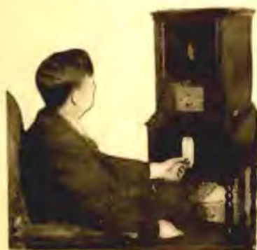
A television receiver which presents pictures eight inches square (R. E. Replogle, assistant to president of Jenkins-DeForest Co.).
