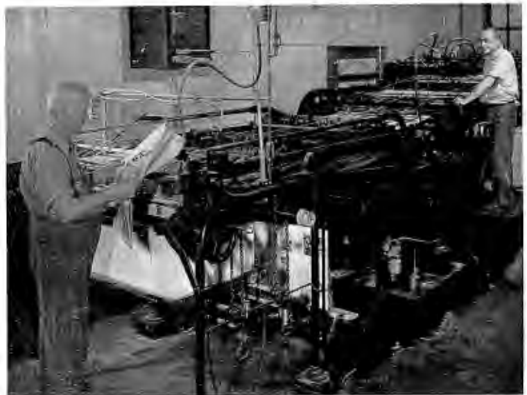
SECTIONS OF this years Family Album were printed on this flat-bed press. John Witcher, left, examines a freshly printed page while Charles Hatak, right, controls speed and feeding of the machine.
