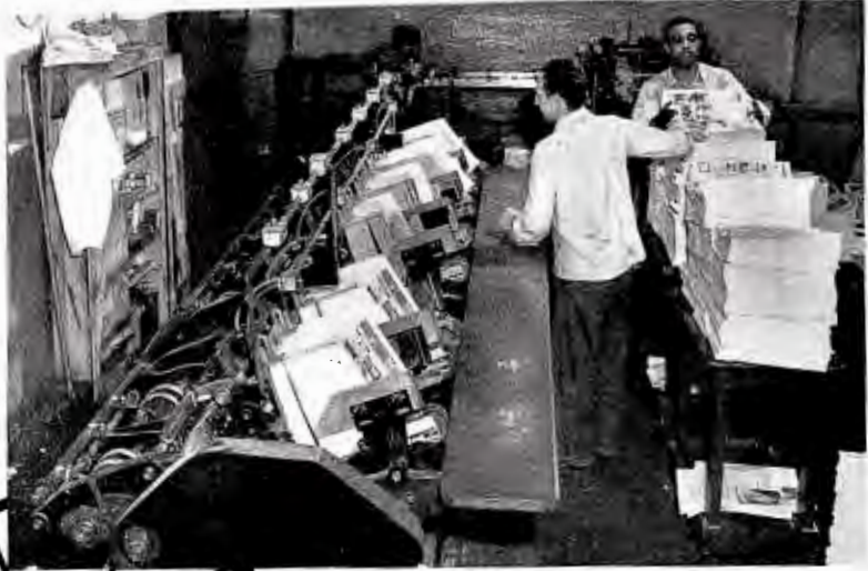
THIS MACHINE assembles all sections of each issue of PRAIRIE FARMER and stitches them together. Ed Papiewis, left, and Julius Nelson feed machine.
