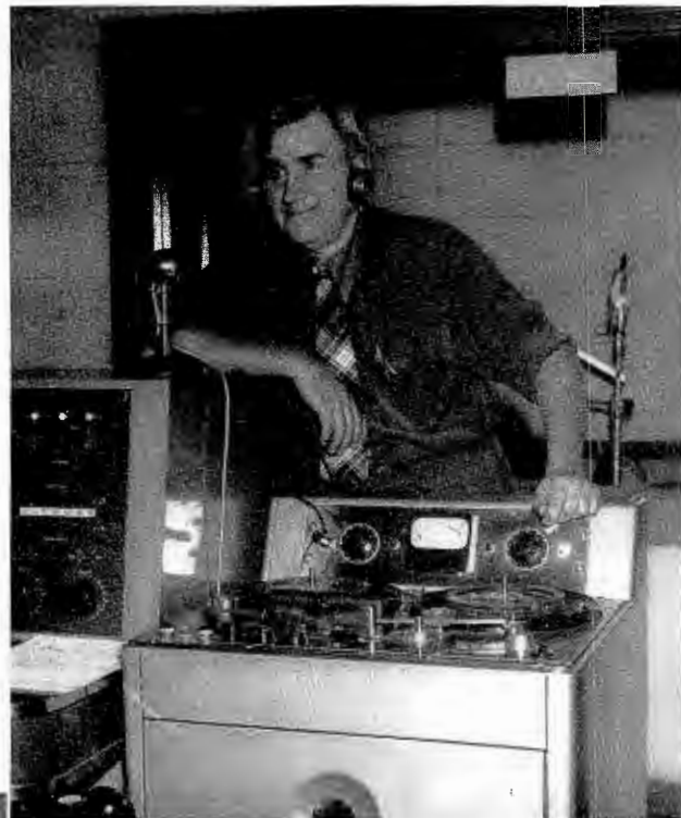
Above, Charles Nehlsen, usually called "Nelly," who spends much of his time supervising the making of recordings. Originally a recording had to be made on a disk or "platter," and many are still made that way. However the tape recorder now gives such perfect results that it equals the natural voice in quality. Words or music are impressed on the tape by magnetic effect, with no mechanical change. The use of recordings gives much greater flexibility in program planning. Nehlsen, a precision worker of great skill, listens to hours of speech and music every day, but is one of the quietest men in the place. Shown here monitoring a control-room tape recorder.
