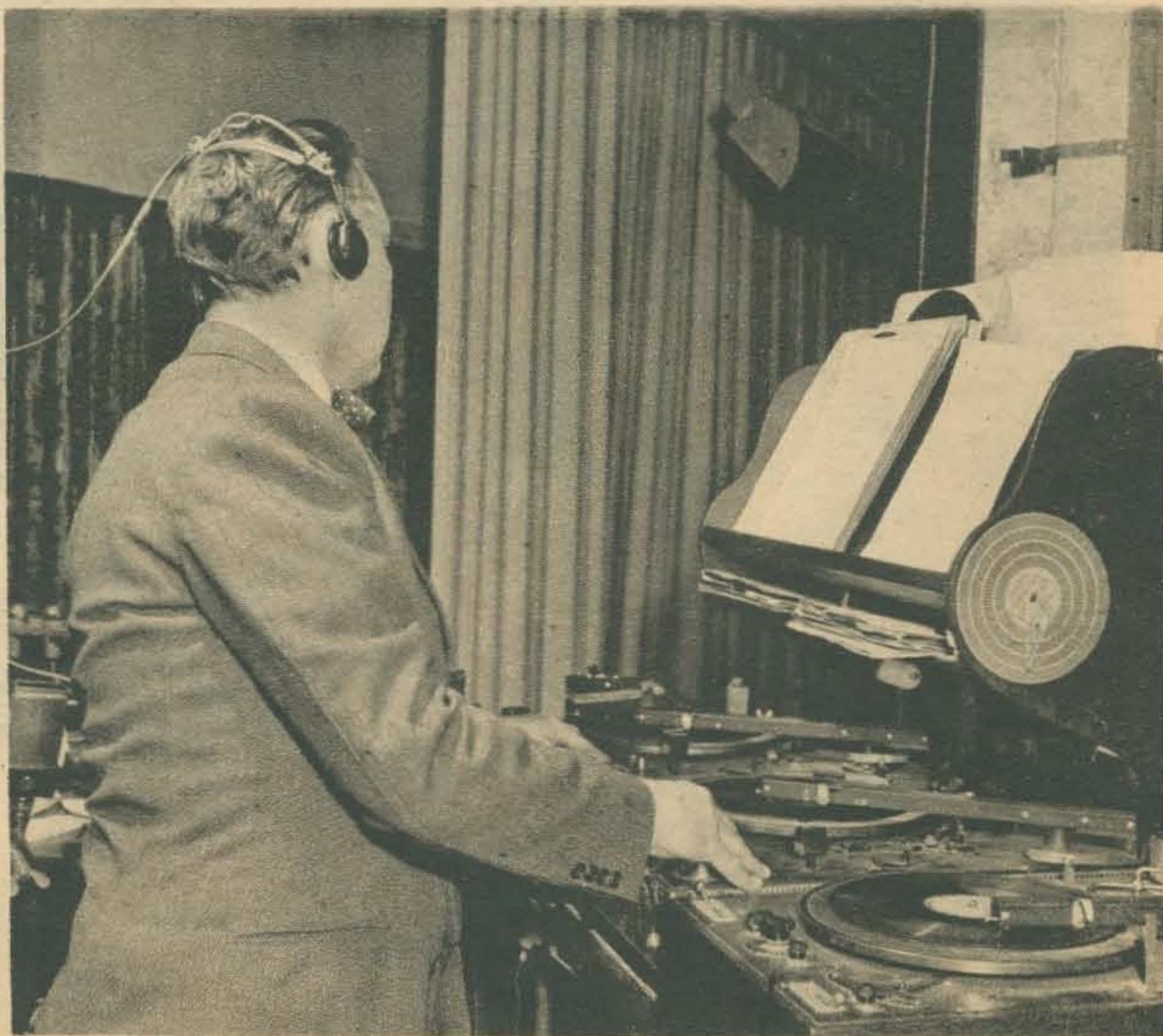
SOUND EQUIPMENT used by Charley Forsyth is among the most elaborate to be found in any radio studio. He operates a battery of three turntables to obtain special recorded sounds
