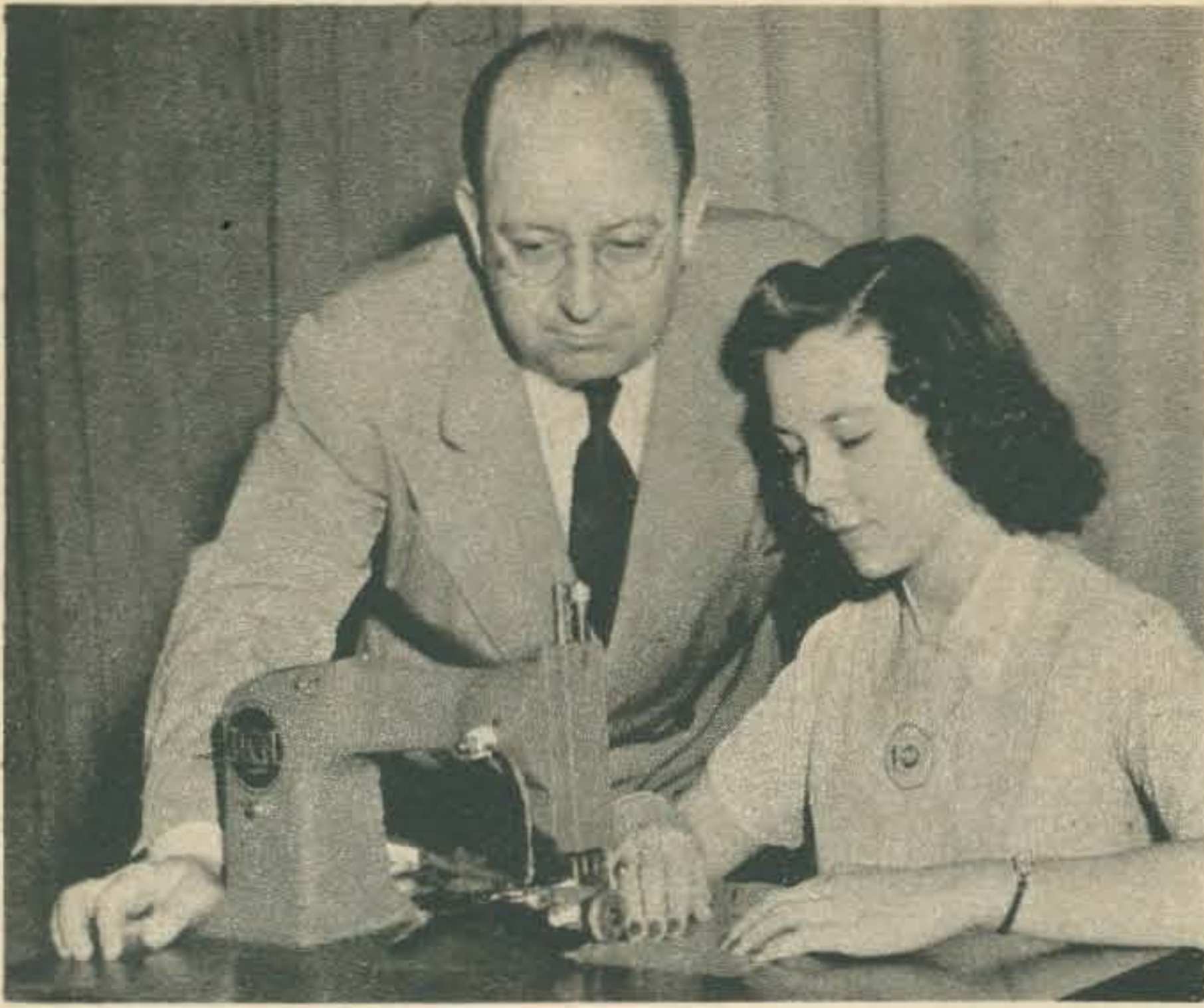
"SEWING" THERMOPLASTICS with radio current instead of needle and thread is demonstrated by Carol Weatherly of RCA, while Dr. George Brown looks on. The thermoplastic-coated material is firmly joined by the generation of heat in the fabric itself.
