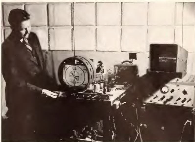
An experimental model of the kinescope—developed by Dr. V. K. Zworykin of RCA Laboratories—is seen undergoing laboratory tests.
