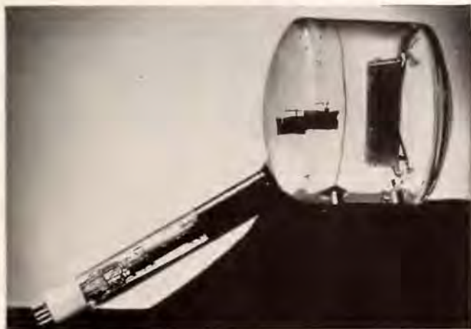
The iconoscope, electronic “eye” of television, invented by Dr. V. K. Zworykin, of RCA Laboratories.
