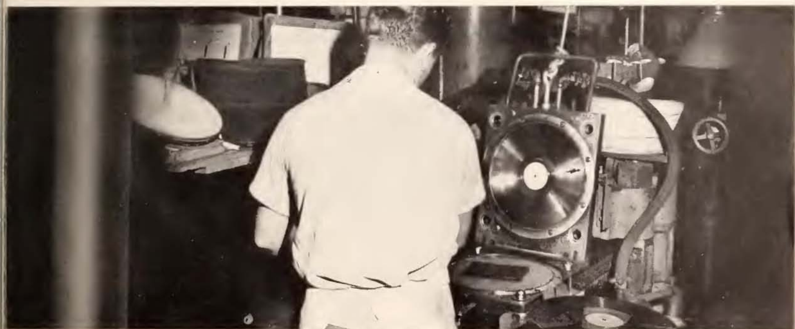
11 - pressing disks is done under great pressure. Transcriptions must be perfectly centered, made under correct climatic conditions, and are usually made of plastic material which resists wear and yet develops no surface noise as needle glides in the groove. High fidelity is possible on transcription
