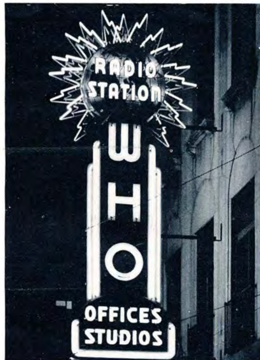
Anyone can read part of this sign. But it takes an expert to know that the flasher on the neon sign is so set that it spells out in Morse code dots and dashes which continually identify the station as WHO.
