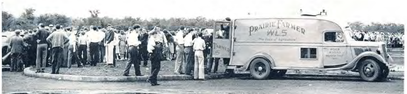
Short wave mobile units WOEB and W9XH, which WLS uses to bring listeners special events programs of unusual interest. This powerful short wave transmitter makes short wave programs possible at a distance of forty miles from the studio.
