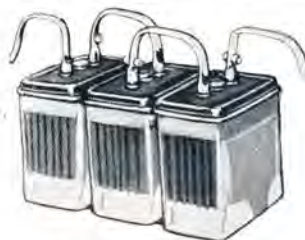
Three 2-volt cells of regular glass jar house-lighting batteries, connected in series, making a 6-volt battery.
