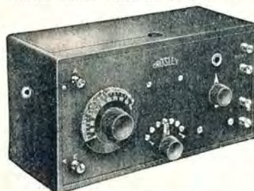
CROSLY MODEL VI. A two tube set that gives uniform satisfaction everywhere. Combines one stage of tuned radio frequency with tuner and audion detector. Price without bulbs, batteries or phones...$28.00
