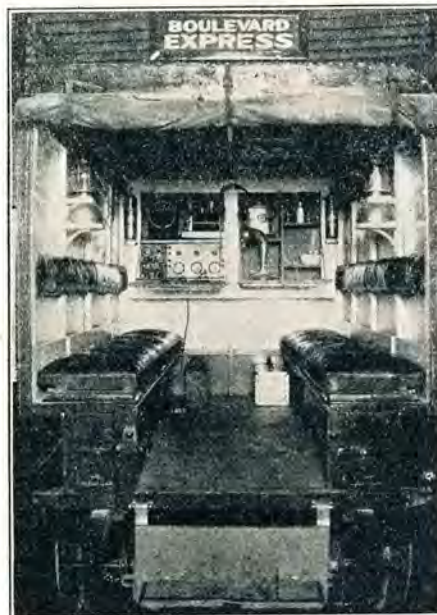
Radio Equipped Trouble Truck
