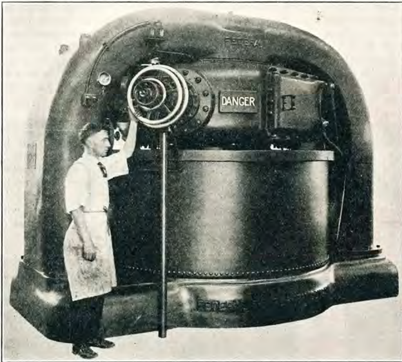
1,000 K.W. arc-converter. The frame and field poles contain 100 tons of soft steel. A station on the Pacific coast for working the Orient is projected, which would employ one of these units, operated on an antenna 1,000 feet high, and expected radiation of 750 amperes.
