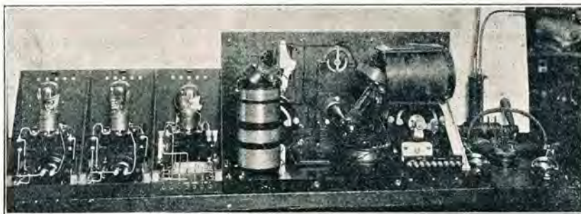
The crystal detector goes into the ash-can! Here is a standard Radio Corporation shipboard receiving set, consisting of a remodelled 106 tuner with regenerative circuit, a detector-tube unit, and two-step amplifier. These instruments replace all cerusite, galena, and carborundum detector apparatus formerly used.
