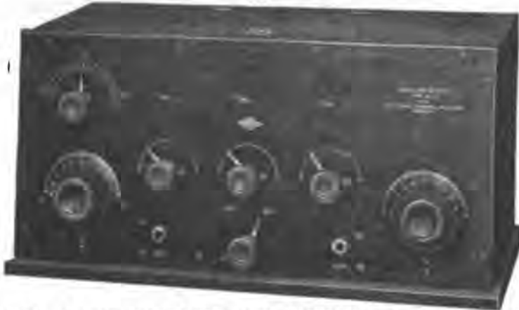
125A—RADIO RECEIVER AND AMPLIFIER.....$125.00 Double circuit, using primary condenser; detector; two stages of audio and one radio frequency. A solid mahogany cabinet. A highly efficient long distance set. Range 200 to 700 meters.
