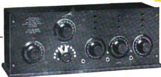
Type AR-2 Receiver Detector and two-stage Amplifier
