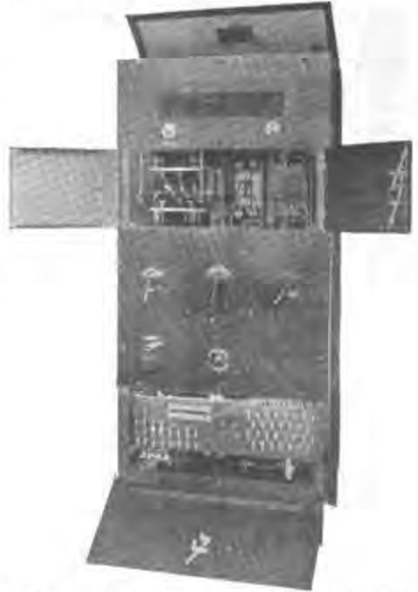
1 K. W. Radio Transmitter Panel for Ocean Telephony. Employing Four 250 Watt Radiotrons as Oscillators and One 50 Watt Tube as Speech Amplifier; Controls Provide for either C. W., I. C. W., or Telephone Transmission on Any Wavelength between 300 and 800 Meters.
