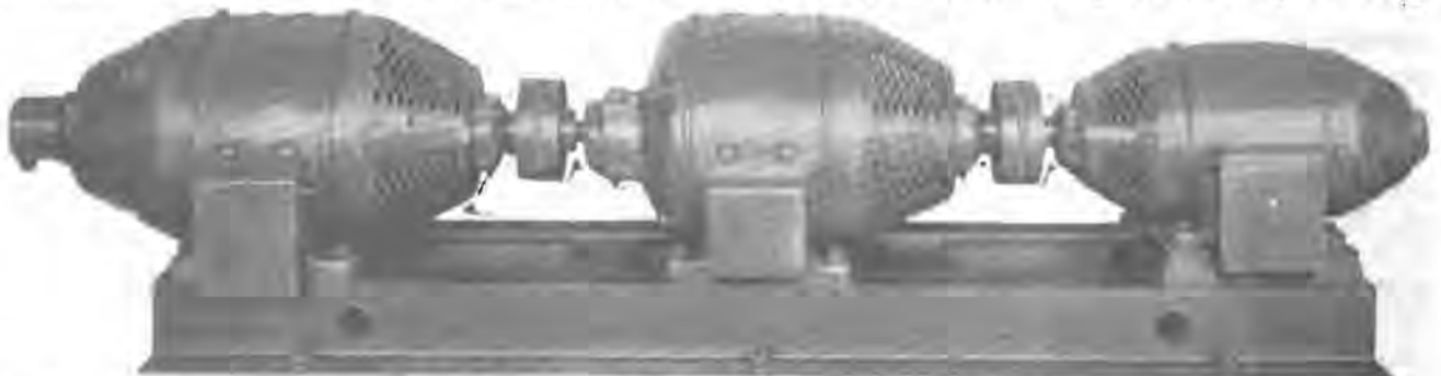
Three Unit Motor Generator Set with 6\frac{1}{4} H. P. 115 Volt D. C. Motor Driving 2000 Volt Generator Supplying Plate Circuit and Double Current Generator Supply 4 Amps. at 125 Volts D. C. Exciting Current and 10 Amps. at 88 Volts A. C. for Feeding 12 Volt Filament Heating Transformer.
