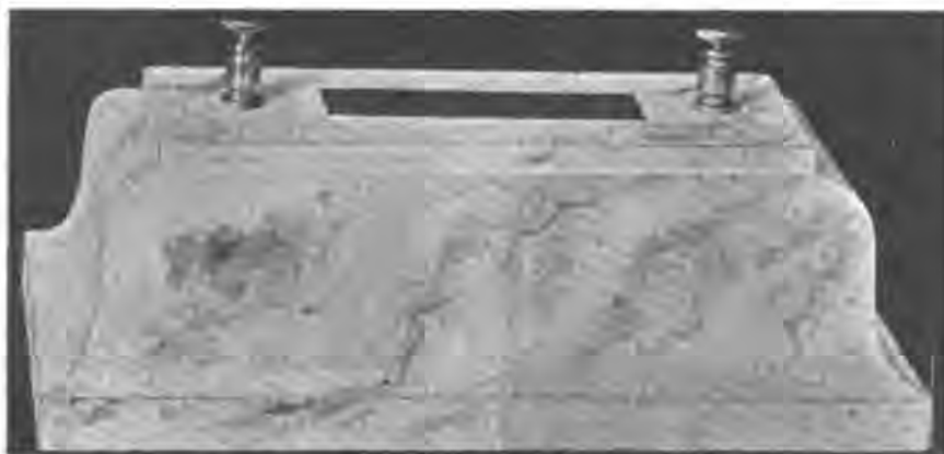
Marble Antenna Invented by W. J. Cormey of Minneapolis To Utilize House Wiring System as Aerial.
