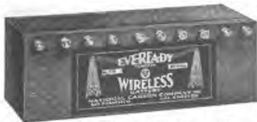
No. 774. The Universal B Battery. One negative and nine positive leads, giving a range of 1½, 8, 4½, 18, 23, 28, 33, 38 and 48 volts.
