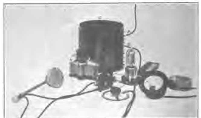
Fig. 25. View of 1/8 Watt Phone Circuit. This circuit utilizes a single receiving tube as an oscillator and can be operated entirely from five blocks of 22 volt B batteries in series for the plate supply and a 6 volt storage battery for heating the filament.
