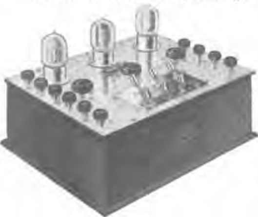
Three-stage power amplifier.
