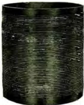
Inductances for transmitters up to 50 watt capacity. 50 turns of wire wound on threaded formica tube. 7 or 26 positive taps. Proper spacing between turns for maximum efficiency. $8.50.
