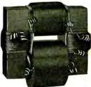
Acme C. W. power transformers. Unmounted. For 60 cycle, 110 volt supply, 3 secondary windings. 6, 12 and 1000 volts, with center tap on high voltage. Designed to furnish 500 volt D. C. when using standard rectifier tubes. Works efficiently with all makes of tubes. $12.50.
