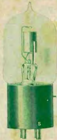
THE A-P TRANSMITTER TUBE —an efficient undamped wave transmitter for use in radio telephony. Price $7.50.
