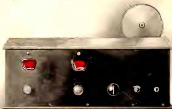
This new circuit design achieves remarkable efficiency with only 4 tubes. Its simplified panel layout is distinguished by glowing spots of light, in place of dials.
