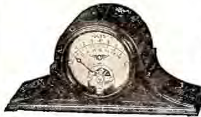
Pat. No. 135-C Portable Voltmeter DeLuxe. Two ranges for checking plate and filament Voltages.
