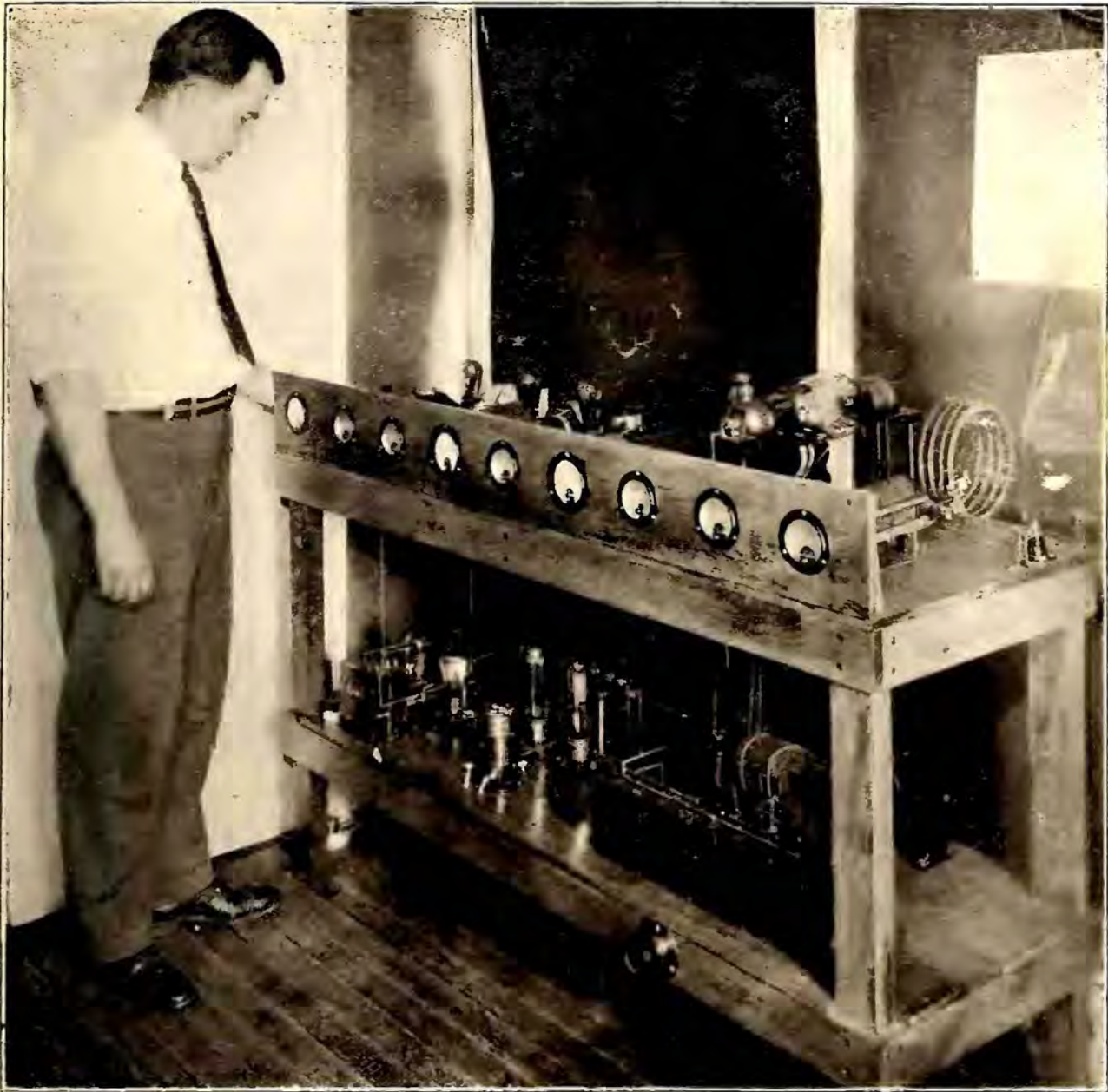
William E. Jackson, Schenectady, and the crystal control short wave amateur transmitter he uses. He, like many other amateurs, is employed during the day, but spends his nights on his hobby. We often wonder when these amateurs sleep
