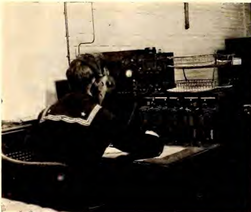
This operator is located at the control station which receives bearings by land wire from compass stations, plots these results and sends the correct bearing to the vessel requesting such service
