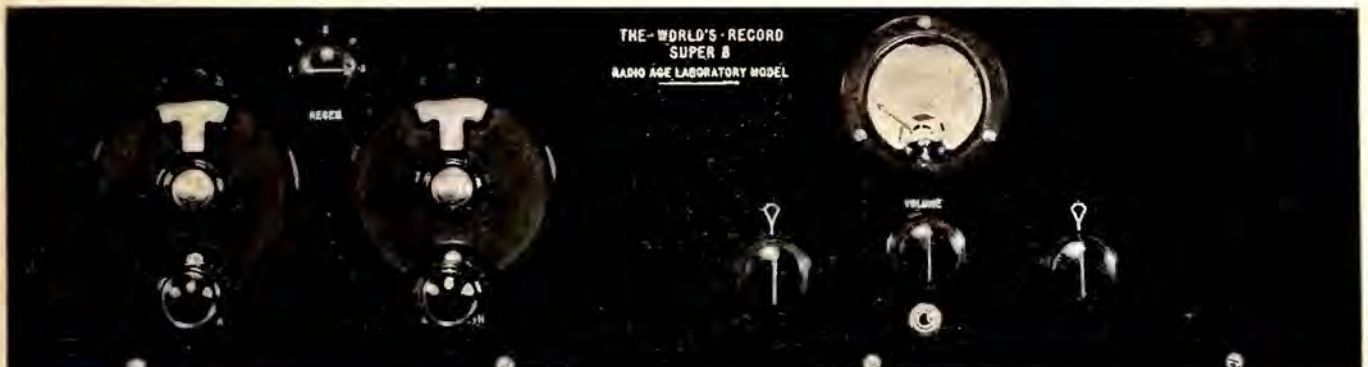
This shows the front panel view of the World's Record Super 8 as modified by Radio Age
