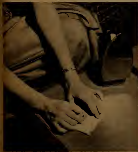
2. She lays a wet cloth over dent, puts an ordinary bottle cap on the cloth right over the injured surface.
