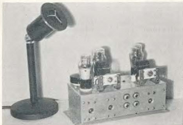
The Radio Frequency section of the miniature transmitter. It is considerably smaller than the "Salt Shaker" mike.
