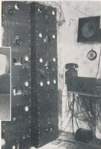
A 30-watt, 56 mc. transmitter and receiver (above) installed in Vermilya's car allows him to operate W1ZE by remote control. The home "shack" contains the extensive up-to-date transmitting equipment shown at the right.
