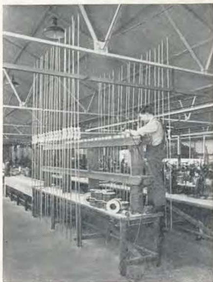
In England where television is already on fixed commercial scale, the demand for receiving antennas has caused tremendous increase in production. The workman above is putting the final touches on special television antennas.
