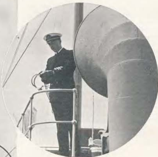
Standing on the bridge, the Captain listens for the fog horns (inset). Noting the time difference between them and the simultaneously sent radio signal, he computes position.
