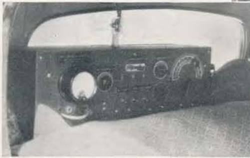
A 30-watt, 56 mc. transmitter and receiver (above) installed in Vermilya's car allows him to operate W1ZE by remote control. The home "shack" contains the extensive up-to-date transmitting equipment shown at the right.
