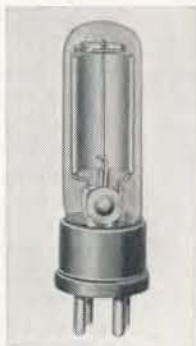
Sound picture photocell. Inside of curved metal is sensitively coated.
