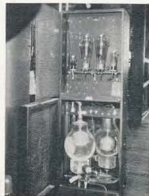
Thyatron photocell tubes used in rectifying large AC currents to DC.
