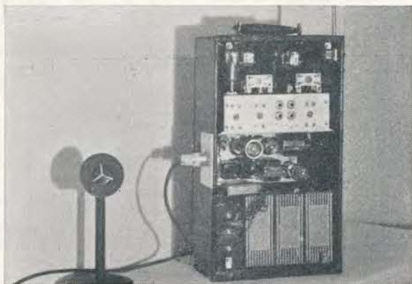
Complete with power supply, the portable rig has an audio frequency response substantially flat to 30-10,000 c.p.s.
