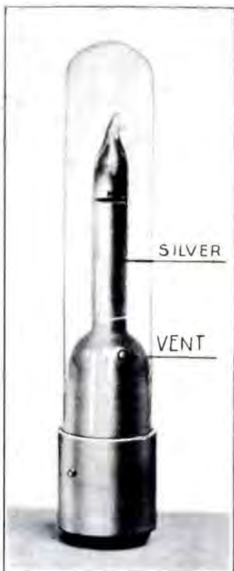
Fig. 8. Type "C" New Donle Electron Tube. It Operates On a New Principle i.e., Electrolytic Conduction of HOT Glass.
