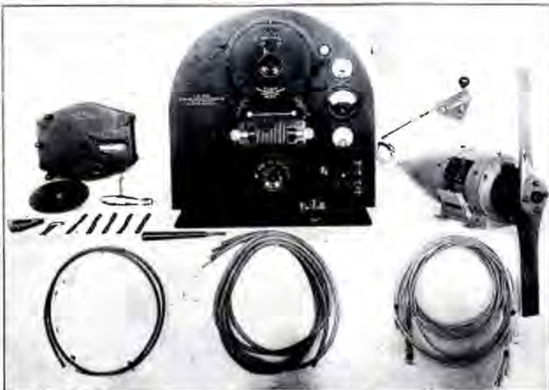
The Air-Driven Generator at the Right is the Contrivance That Supplies the 500 Cycle "Juice" for the Transmitter. The Airplane Therefore Literally Uses Wind to Send With Great Stuff!
