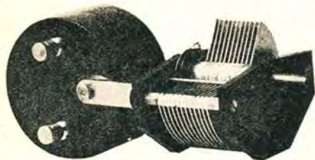
NEUTROFLEX TRANSFORMER Mounted on Kilbourne and Clark Condenser
