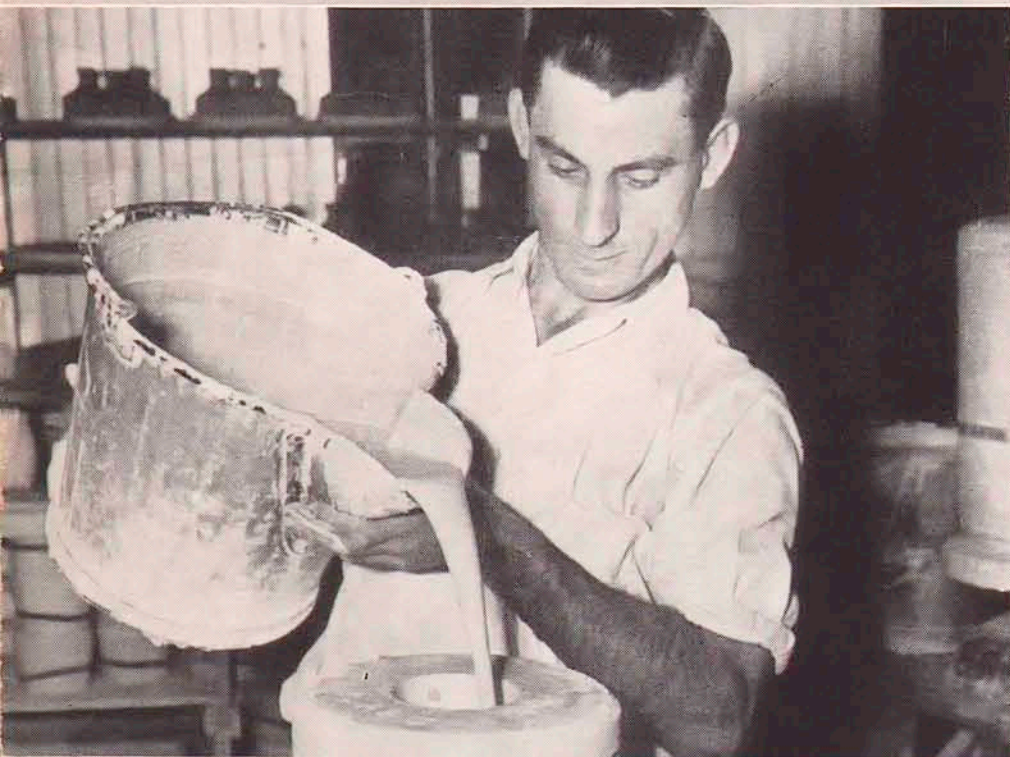
POURING VASE MOULDS in the hot, moist air of a Trenton, N. J., factory, this man is one of America's 167,000 pottery workers, thirty percent of whom are women. The potter's job, listeners learned, was old before Bible times
