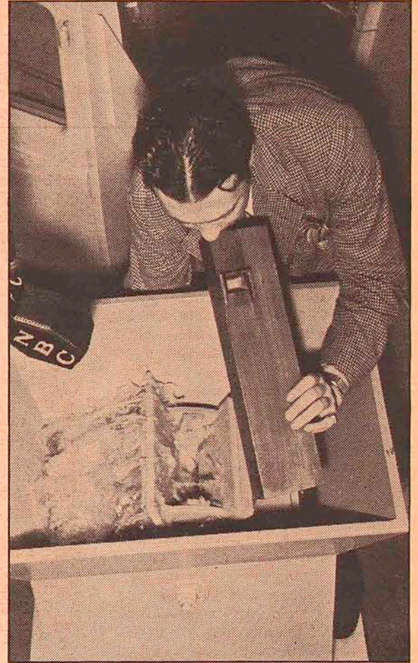
Conjuring up a heavy fog at sea is simplicity itself, requiring nothing more than a paddle-wheel churning water in box, and the wooden-box fog-horn which Saz (above) blows as he turns wheel
