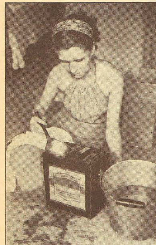
11. Miss Whitaker fills air-cell A battery. Rural electrification is scarce, but listeners are proud of elementary battery sets
