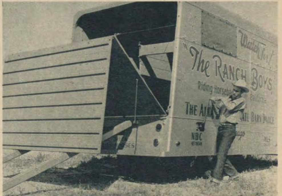
Compartments in the truck carried all essential equipment, and the ramp Ross is lowering above permitted horses to get in and out without danger. Three bales of hay, six sacks of oats and 150 gallons of water were carried for horses constantly
