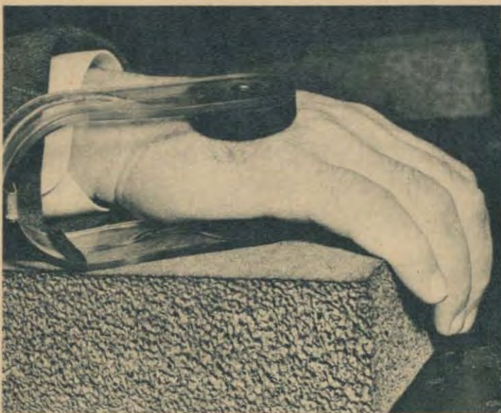
To record the "brain waves," or electrical nerve-impulses set up by fear—the emotion recorded by the psycho-detectometer, electrodes are clamped to hands and at the base of the brain. Some "lie detectors" are based on blood-pressure, perspiration, other reaction indicators
