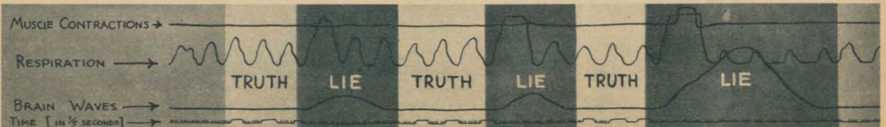
To record the "brain waves," or electrical nerve-impulses set up by fear—the emotion recorded by the psycho-detectometer, electrodes are clamped to hands and at the base of the brain. Some "lie detectors" are based on blood-pressure, perspiration, other reaction indicators
