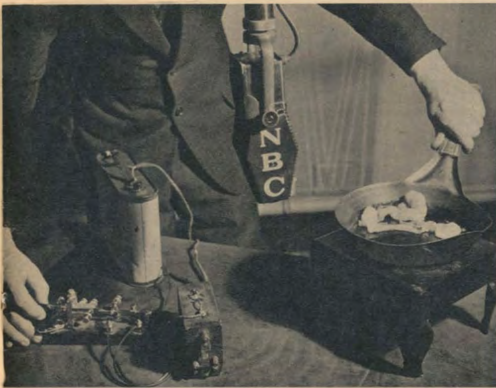
Electrocution of a human in Karloff dramas is achieved by radio technicians with a frying-pan of bacon sizzling on an electric grill plus the sound of flying sparks obtained from an ordinary telegraph key and dry-cell battery
