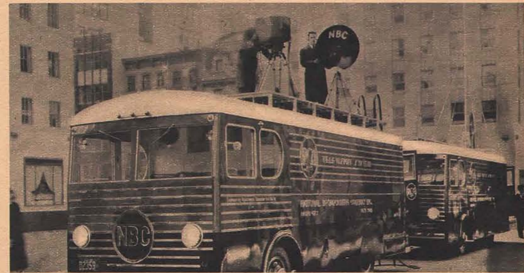
27 First American mobile television unit belongs to NBC and is being used in experimental pick-ups of outdoor events. In the first unit are cameras and microphones; in the other van is the transmitter, connected by cable. The broadcast is thus made directly from the spot
