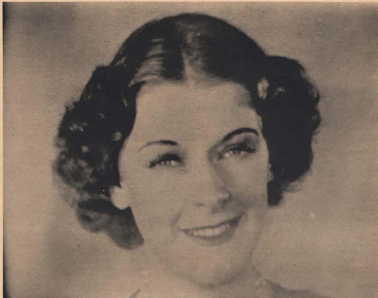
9 The more scanning-lines, the clearer the picture, as was shown in the pictures at left. Above is the image of Betty Goodwin, NBC television announcer, as she appears on a 343-line screen in actual transmission
