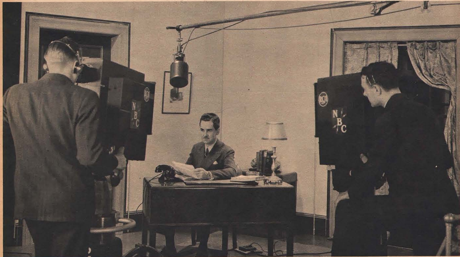
17 Television and sound-broadcasting are sometimes similar in many ways. In both instances, Lowell Thomas works seated at a desk. In sound, the microphone is set on the desk. In television it hangs on a hook out of
