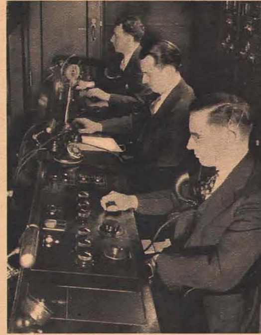
23 An engineer (foreground) monitors sound; one (rear) monitors picture. The program director faces the "talk-back mike"
