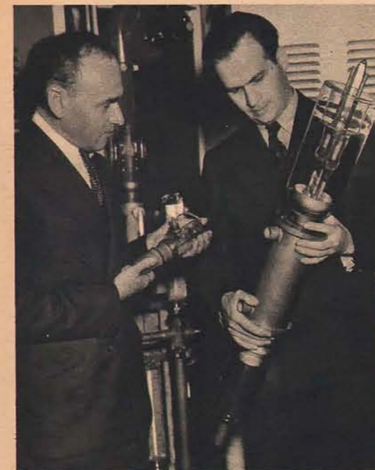
28 Gilbert Seldes and Dr. Peter Goldmark of CBS inspect the largest (15,000-watt) and the smallest (100-watt) water-cooled tubes
