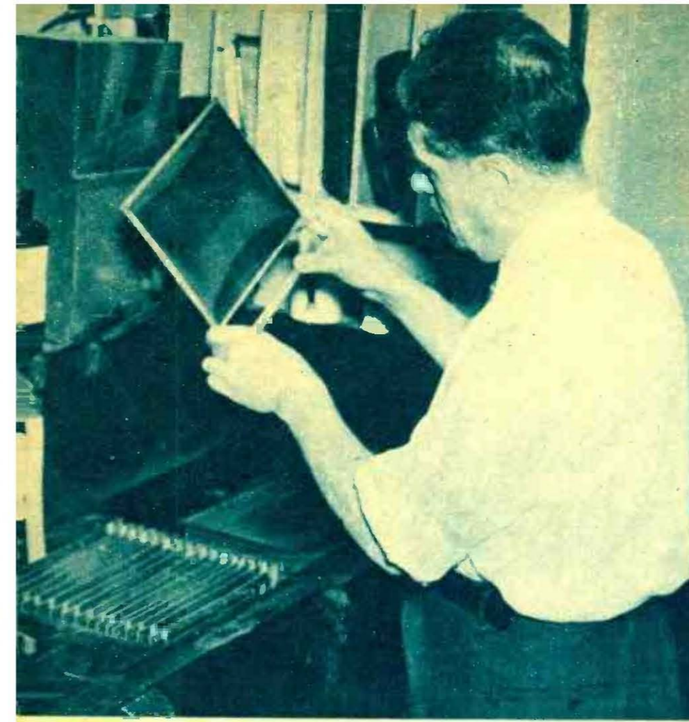
9 After the picture-taking is completed, the negatives are developed by Paul Kirsch, then put into a hypo bath. This process takes thirty minutes
