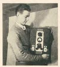
One of the Smoky Rangers is proudly displaying a new model 15-watt combined transmitter and receiver designed for portability
