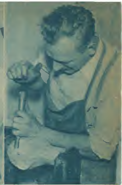
7 The next step is to hollow out both halves of the head. Again Frank uses the hand chisel
