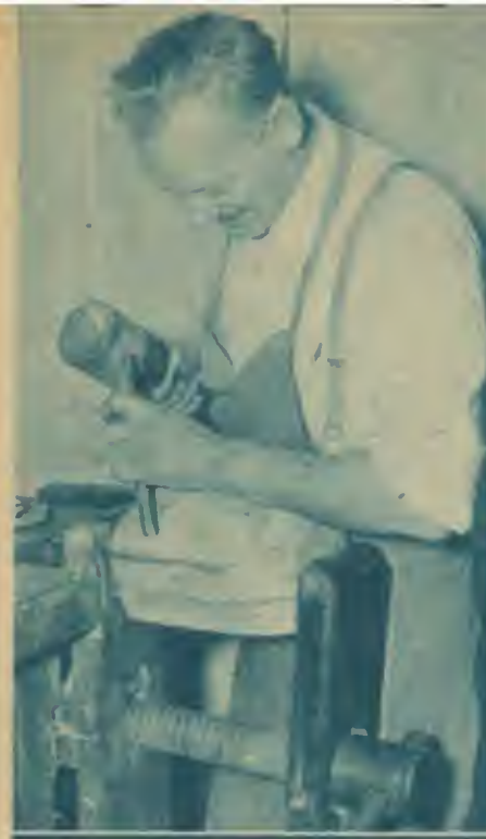
4 Using a mallet and a heavy chisel, Marshall then does the rough carving of the head
