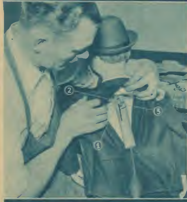
16 Lever (No. 1) and the bulb control the mouth movements, cord (No. 2) works the winking eye, ball (No. 3) rolling eyes
