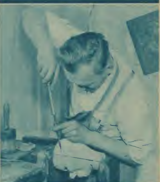
9 When all movable effects have been put in the head of the dummy, the two halves are screwed together again
