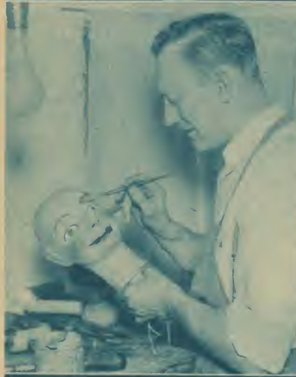
10 The head is then given four coats of a special paint Frank mixes himself. It's sanded between each of the first three coats
