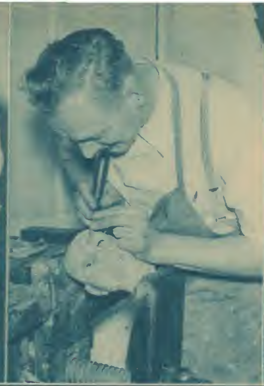
5 Using regular wood-carver's tools, Frank finishes the face of the dummy with hand chisels, sandpaper
