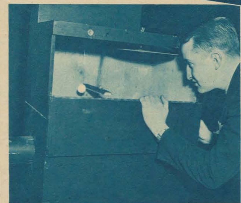
Ray Kelly takes a look into his rain machine. Above the box is a hopper filled with bird-seed. The seed drops down onto the disk, which can be seen on a level with Kelly's head. A wind-shield wiper brushes it off to fall on a triangular shaped board which scatters it. The seed then falls onto several surfaces of different height, rattles on the ping-pong ball!
