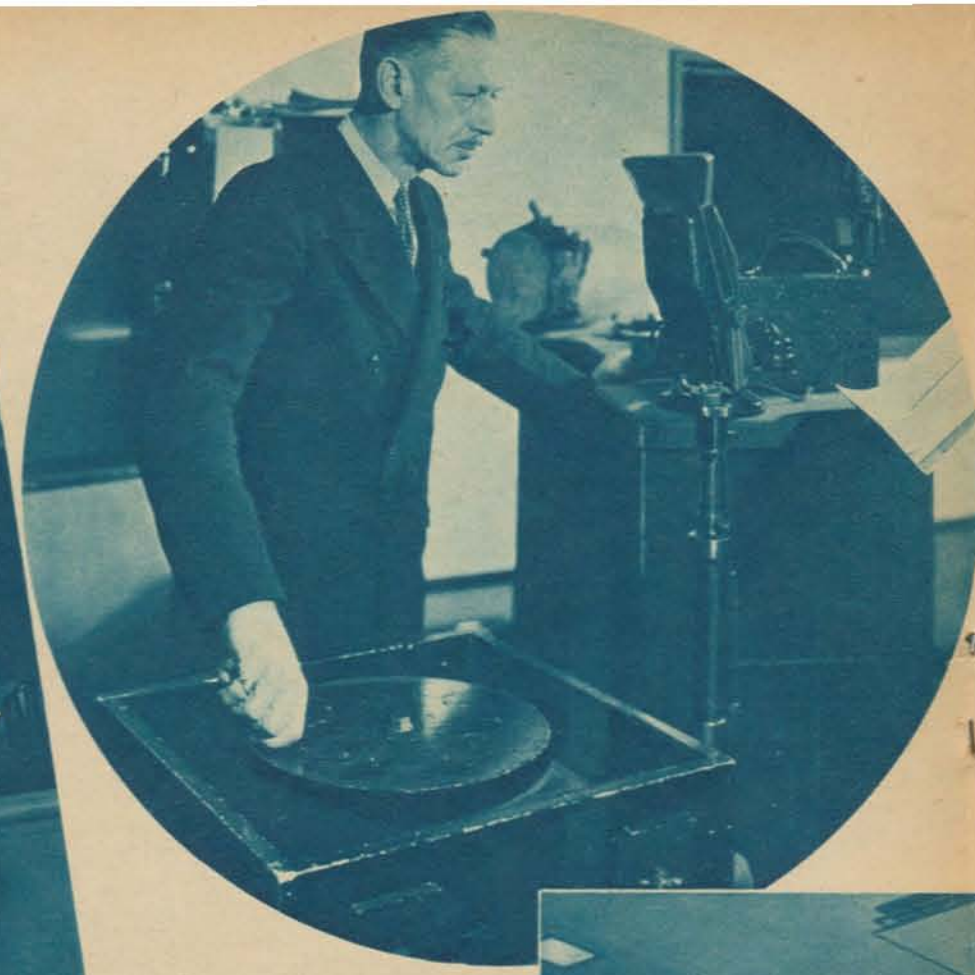
Above: Here Engineer Al Van Brakle of Columbia's sound-effects department produces the sound of a railroad car, vintage 1880. He's using a heavy iron disk on wheels, rotating it rapidly to make the clickety-clack, clickety-clack of an old-time railroad car bumping over a rough track
