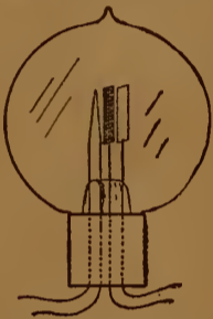
Figure 45—The De Forest vacuum tube, showing the minute screen placed between filament and plate
