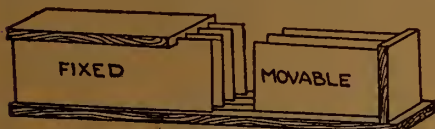
Figure 37—An early form a variable condenser, bulky, mechanically bad and soon discarded
