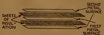
Figure 36—The second step toward compactness and greater capacity for a given plate area
