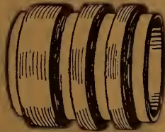
Figure 19—Bank-wound coil divided into sections
