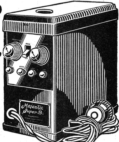
The Majestic is connected to your radio just like "B" batteries and attached to an ordinary electric socket. (For 1 to 12 tube radios.) Replaces "B" batteries entirely and furnishes "B" current direct from regular house lighting current. Simplifies radio receiving. More efficient than dry or wet "B" batteries. Entirely noiseless. Operates from 110 120 AC, 50-60 cycle current.
