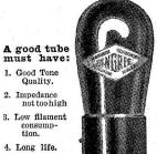
Pingree Tube Characteristics Plate imped-ance 8500 — 10,000 ohms. Amplification factor 8-9. Filament con-sumption .25 amp. Filament volt-age 5.0 volts.
