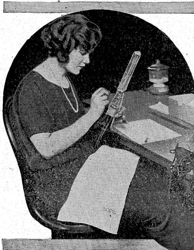
A girl's deft fingers formed the tongue with which S. S. Leviathan "speaks" at will by Radiotelegraph to either side of the ocean. Miss Marie Fencil is assembling the "tongues" of the 10,000-watt vacuum tube. Two of these furnish the power to the Leviathan's big Radiotelegraph transmitter which has power enough to span the Atlantic. Western Electric Photo
