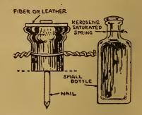
tle where it is to be cut off. Light the string and in burning the string it heats the bottle neck. When the fire is burned out, simply plunge the bottle into cold water and then tap the bottle lightly and your insulator will fall right off, cut neatly where you tied your string. I have made as many as ten of these in as many minutes and they are as efficient as those that are purchased.—B. P. Craig, Youngstown, Ohio.
