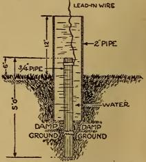
Secure a piece of galvanized pipe % inch in diameter and 5½ feet long, also a piece of 2 inch pipe 3 feet long. Drive the % inch pipe into the ground about 1 foot. Fill the pipe with water and let it settle, then fill it up again. The water in the 2-inch pipe serves to keep the smaller pipe full all the time and also keeps the ground wet around the smaller pipe.—Dick H. Roberts.
