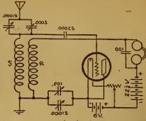
same as a one tube for local. The colls represented are the rotor and stator of a variometer.—Fritz Franke, Chicago, Ill.
