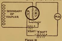
tial will again cause a further increase in the plate circuit current, for more electrons are being emitted at the higher temperature.
