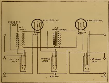
Figure 1-Wiring Diagram for Amplifier
