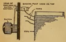
knurled set screw head is used for the switch points. The base, which is back of the panel, is used for the connection and it may also be held with the screw for attaching the binding post to its base.—Chester Wilson, Chicago, Ill.
