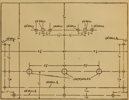
Figure 2-Panel Layout for Amplifier
