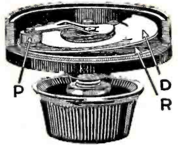
This shows the exclusive rocking disc construction of Centralab volume control. "R" is the resistance. Contact disc "D" has only a rocking action on the resistance. Pressure arm "P" together with shaft and bushing is fully insulated.
