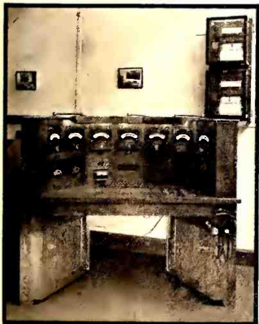
Special bridge used in the Van Cortlandt Park Laboratories for measuring the electrical characteristics of radio vacuum tubes
