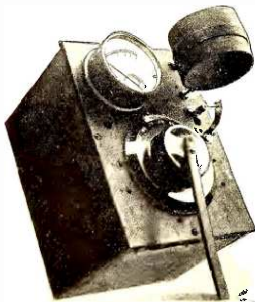
Fig. 1—External view of home-made wavemeter. The resonance indicator is a d.c. milliammeter.
