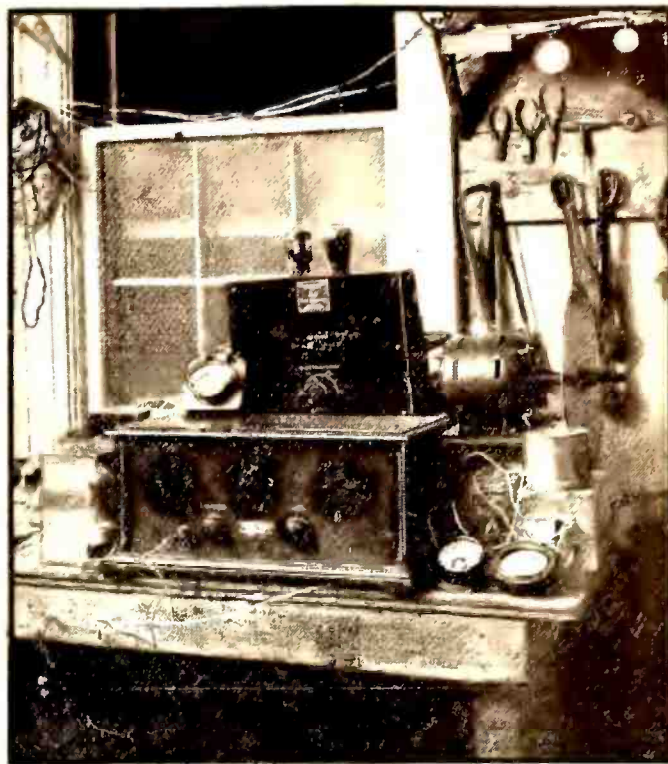
A close-up view of the transmitting scanner and television amplifier
