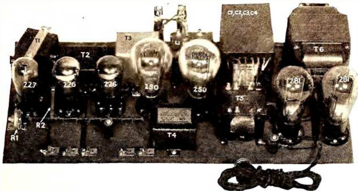
GENERAL VIEW OF PUBLIC ADDRESS AMPLIFIER
