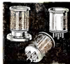
New 5-prong plug-in coils, for short and broadcast waves. Wound on forms of threaded, moulded bakelite.
