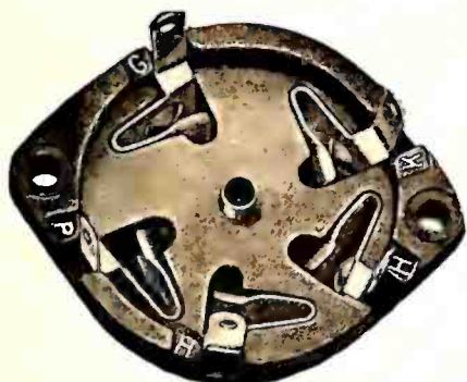
Bottom view without base showing contacts
