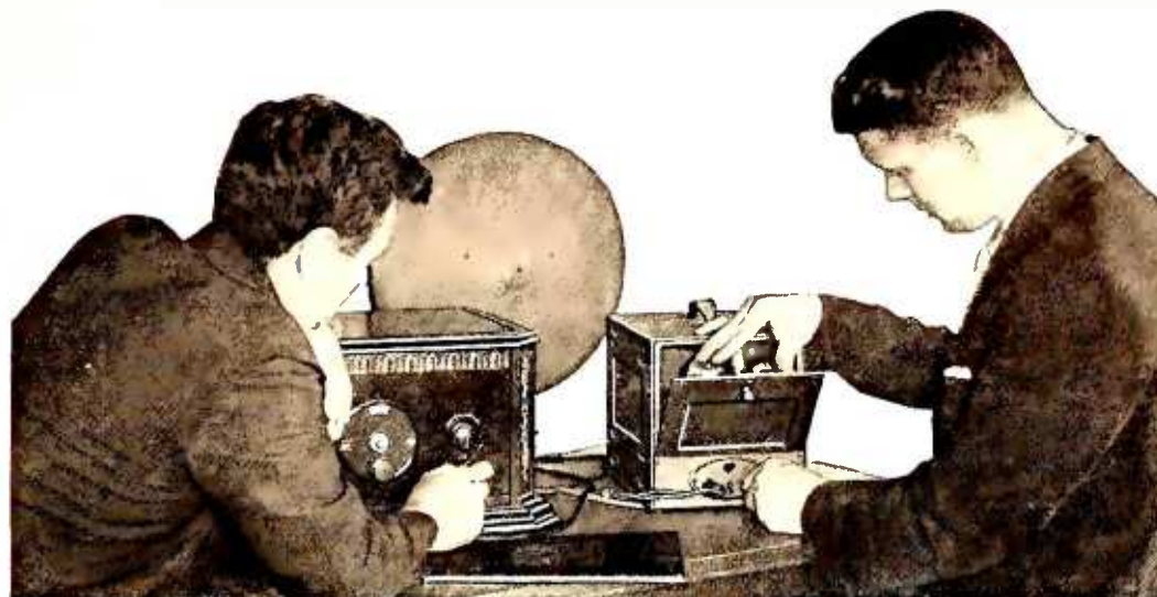
A radio set of other years can be brought up to date by improving the audio quality through new transformers, tubes and loud speakers or by the purchase of a complete power-supply-amplifier unit. These changes help greatly. R.f. Changes are not suggested
