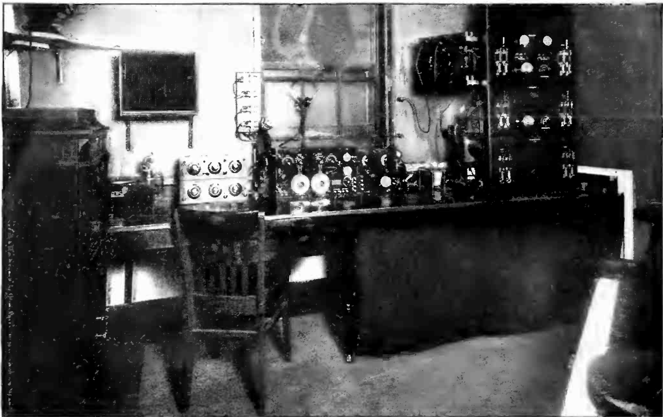
WGI, THE AMERICAN RADIO & RESEARCH CORPORATION'S STATION AT MEDFORD HILLSIDE, MASS. The 100-watt transmitter, shown at the right, has been heard in Kansas, Texas, and Cuba
