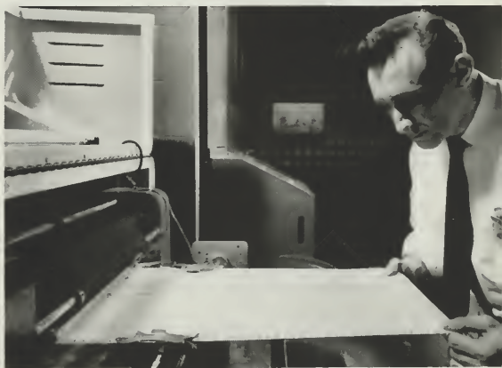
6. When Computer finds a depot short of an item, it passes information on to Electro-Mechanical Printer which prints re-order form at 600 lines a minute.
